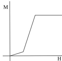
**Fig. 1.** Ideal primary magnetization curve
