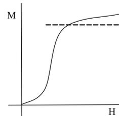
**Fig. 2.** Real primary magnetization curve
