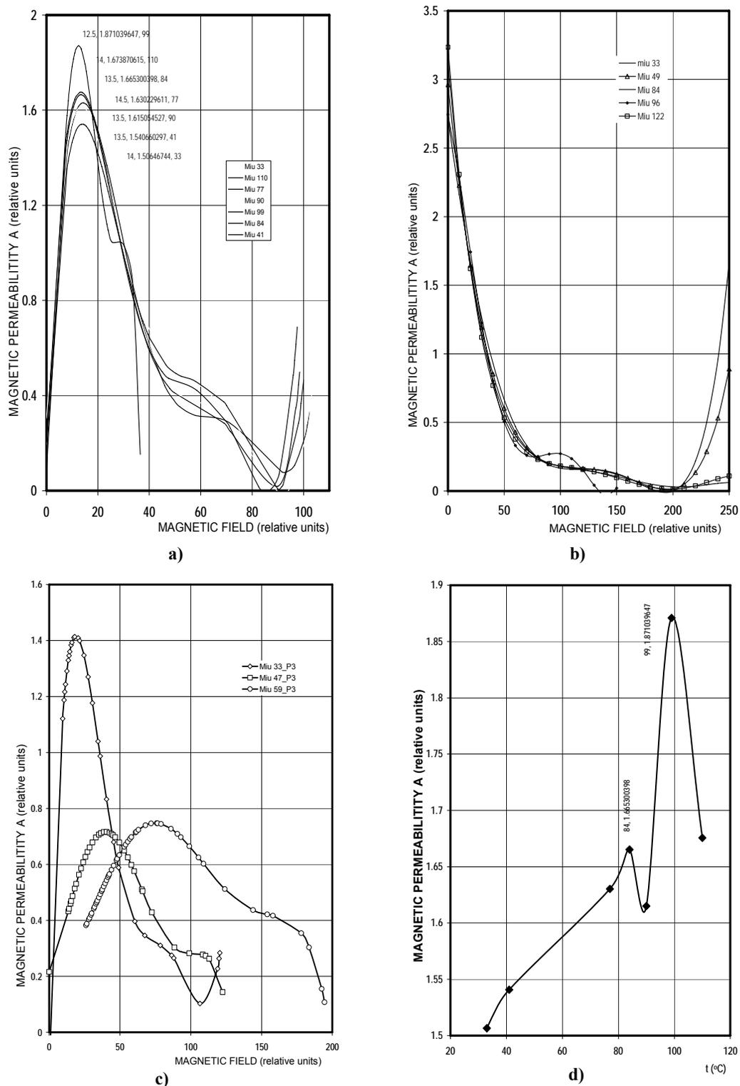
Fig. 6. The Stoletov curves dependency by the temperature for studied samples
