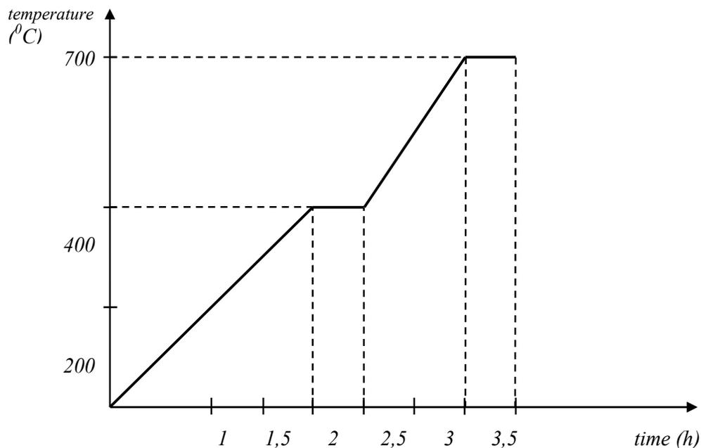
Fig. 2. Chart time-temperature of the pyrolysis process
