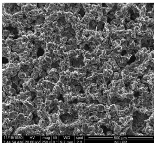
**Fig. 3-7.** SEM images of various samples of PAN and NaCl with details from the size of 50µm up to 500µm
