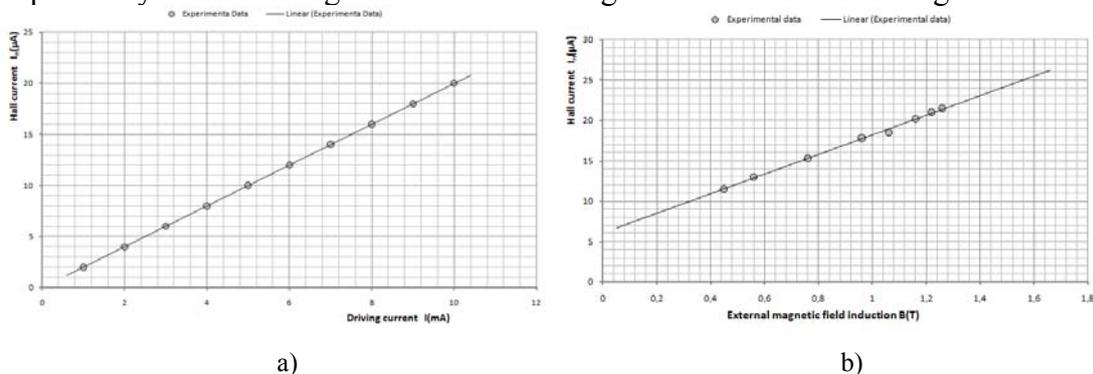
**Figure 2:** The linear dependency of Hall voltage on the external magnetic field and the driving current
