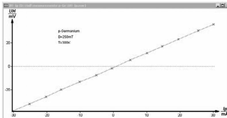
Figure 4: The Hall voltage as function of the current
