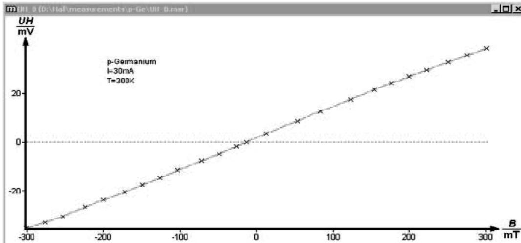
**Figure 6:** The Hall voltage as function of the magnetic field
